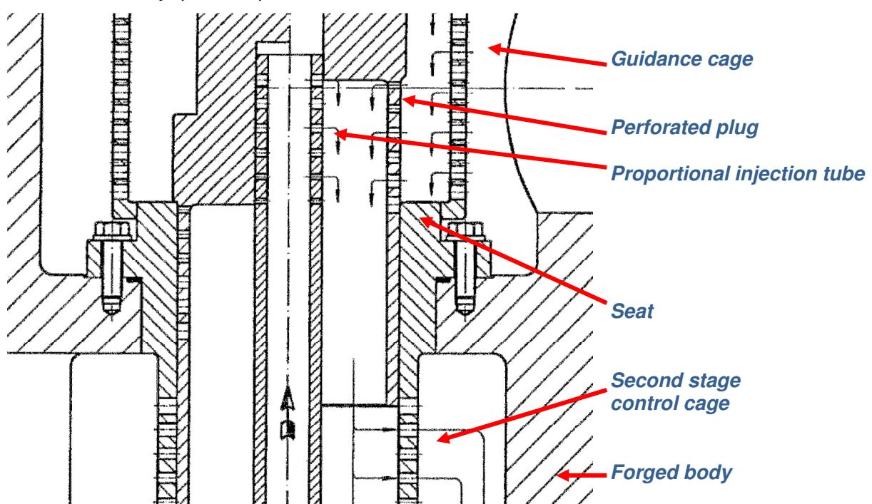
This trim design is used in forged body designs as well as in cast valves. The advantage is the optimal mixing of the cooling water into the steam. The water pressure drop creates small droplets, injected in the most turbulent part of the valve, followed by cages and throttling plates.
