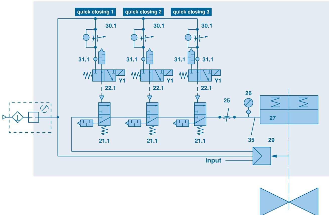
*Schematic showing a quick closing device based on EN 12952-3 / TRD 421. The 3 quick pneumatic valves discharge the air from the “spring to close” pneumatic actuator and are also closing the air supply from the positioner when the quick closing valves are activated.*
