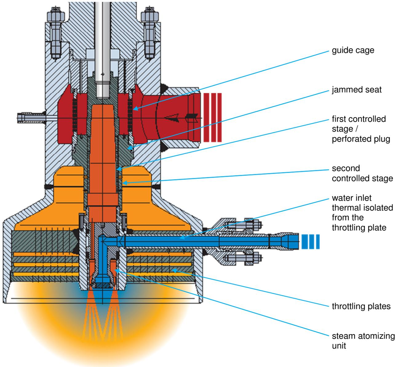
In the show valve above we see a 6 stage pressure reduction, based on 2 controlled stages and 4 throttling plates. The steam cooling is done with a steam atomizing unit, positioned in the centre of the valve.
