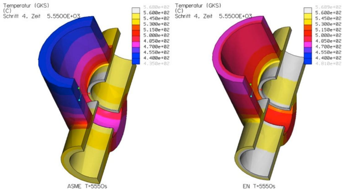
Comparison of a valve to **ASME 16.34** with a valve designed to **EN 12516-2** is available on request.
