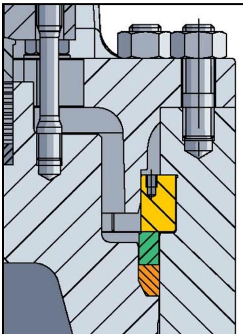
In our experience a regular pressure seal is hard to open. The split ring is held in place by the bonnet, and the bonnet has to be driven down to remove the split ring. Due to corrosion, magnetite and the tolerances this is not always easy.
