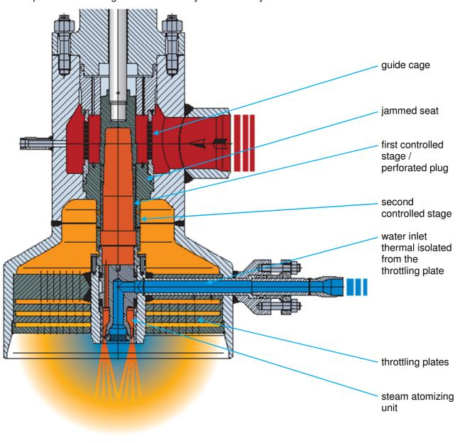
In the show valve above we see a 6 stage pressure reduction, based on 2 controlled stages and 4 throttling plates. The steam cooling is done with a steam atomizing unit, positioned in the centre of the valve.
